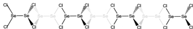
Fig. 4 Illustration of the two crystallographic sites available for the Se atoms of \text{Se}_2\text{Cl}_4^{2-} in compound 5 . Note that the Cl positions are fixed. The sites in grey are occupied by 10% of the Se–Se units in the structure, the black sites are occupied by the remainder.
